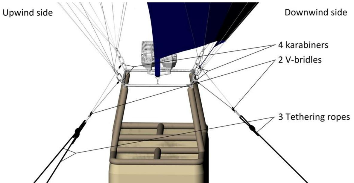
Picture 1: Parts for the tethering system
