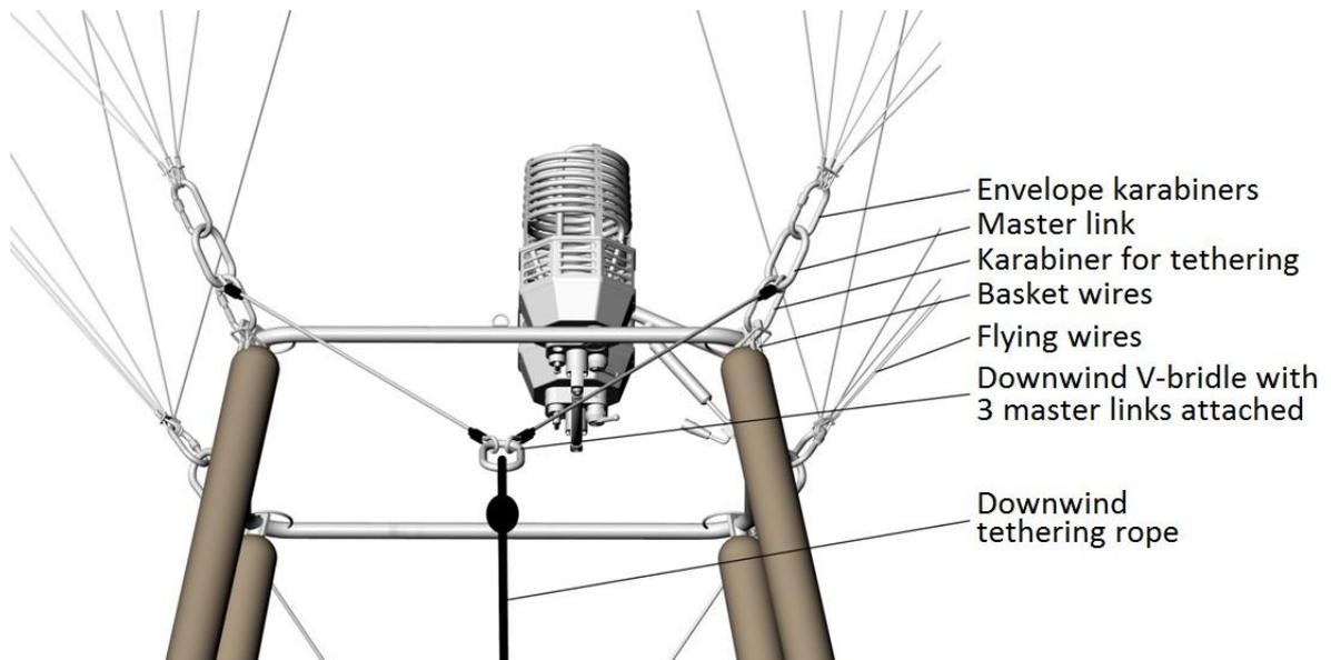
Picture 3: Downwind assembly
