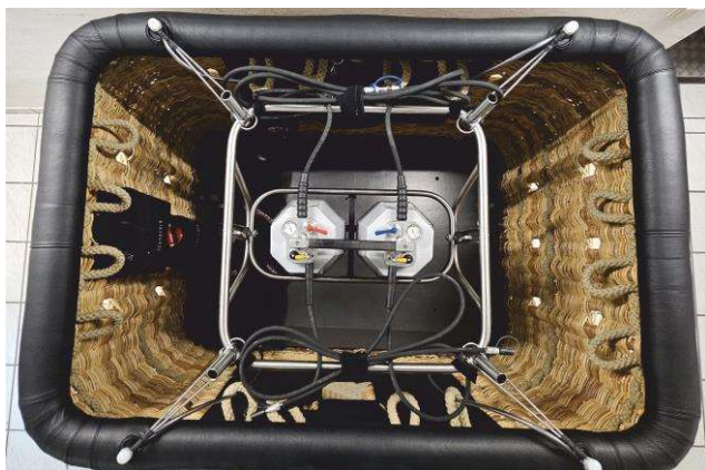
5-3: Ground handling burner
