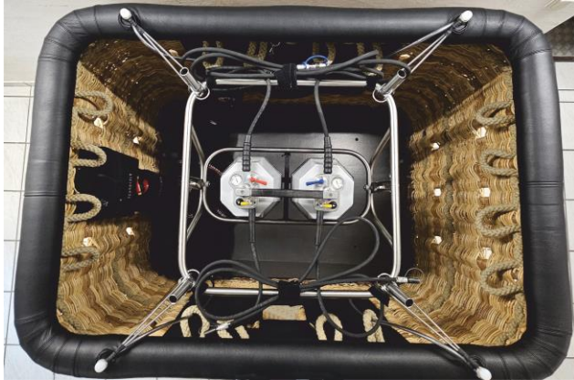
5-3: Ground handling burner
