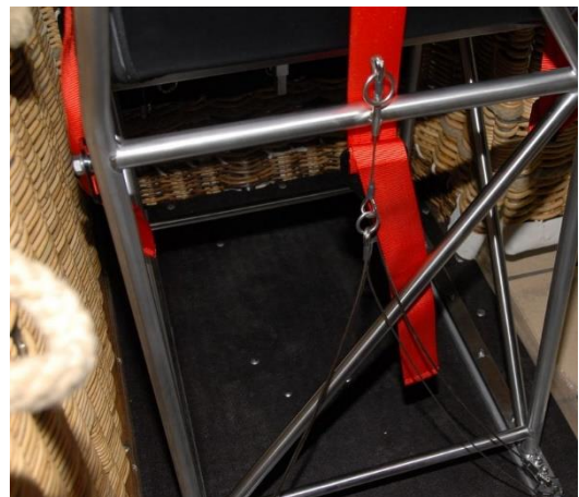
Image 2: Deactivation of the safety bolt
