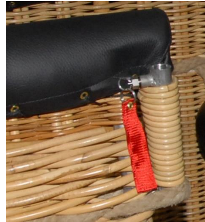
Image 6: Locking pin of the door
