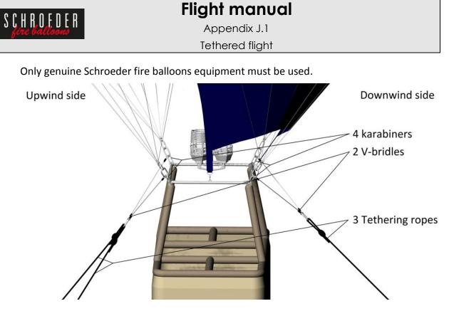
Picture 1: Parts for the tethering system
