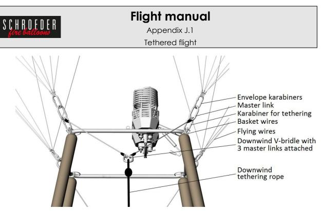
Picture 3: Downwind assembly
